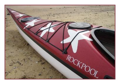
It has a clearly visible V through its entire length and a soft chine edge in the midsection that blends smoothly before reaching bow or stern.
