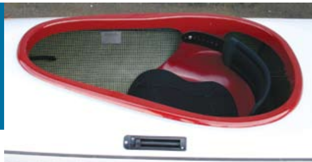
The back band can be adjusted by removing the bolts that attach it to the seat hangers.
